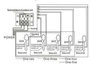
IMPORTANT: Connect the connective cables to the terminals as identified with their respective matched numbers on the terminal block of indoor and outdoor units. For example, see the following US models: Terminal L1(A) of outdoor must connect with terminal L1 on the indoor unit.
