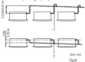
T-joint converging drain pipes
