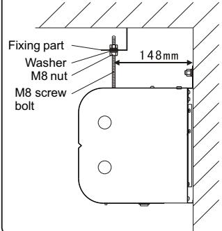
4. After fix the air curtain, connect the water inlet tube and drainage tube (offer by user), ensure without leakage of water.
