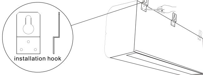
2. For install on the concrete and brick wall or other hard wall, should measure the place of the installation screw (see the "installation dimension"), then fix on the wall by M8 expansion bolt, ensure the out expansion bolt around 13-15mm.
