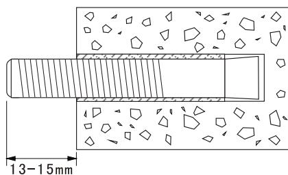
3. Ensure the expansion bolts are fixed and hang up the air curtain, and then fasten the screws.
