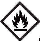
A2L | <b>WARNING</b> | This symbol shows that this appliance used a flammable refrigerant. If the refrigerant is leaked and exposed to an external ignition source, there is a risk of fire. |
