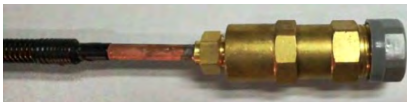
Figure 7.7D – Plastic Seal Removal
