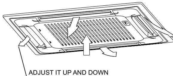
While this function is set, the swing fan of indoor unit runs; otherwise, the swing fan doesn't run. The swing scale of every side is 30°. When the air conditioner isn't in operation (including when "TIMER ON" is set), the **SWING** button will be disabled.
