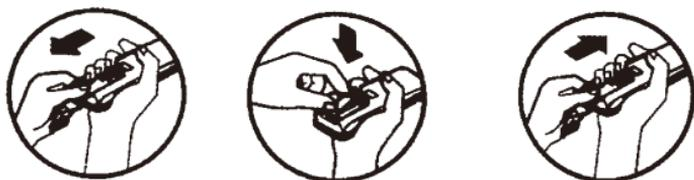
Slide open the cover according to the direction indicated by arrowhead.
